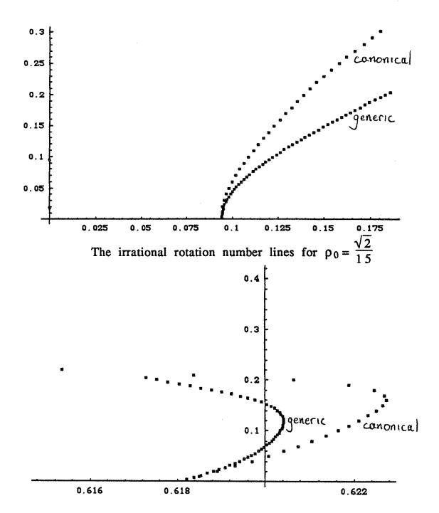
These plots correspond to rotation numbers  $\frac{\sqrt{2}}{15}$  and the golden mean, or  $\frac{\sqrt{5}-1}{2}$ . In both cases the more generic function is the more densely plotted line. The data for the canonical map has been condensed along the a axis so that the invertibility points (the value
